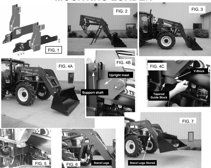
**STEP 1** For a new loader installation, the mountings must be installed on the tractor first. Refer to the typical mounting kit shown in Figure 1. A detailed schematic of your specific kit is available—just call 1-800-570-8205 if the schematic was not included with your new loader.
